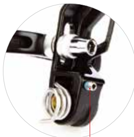
Balance spring power adjustable
